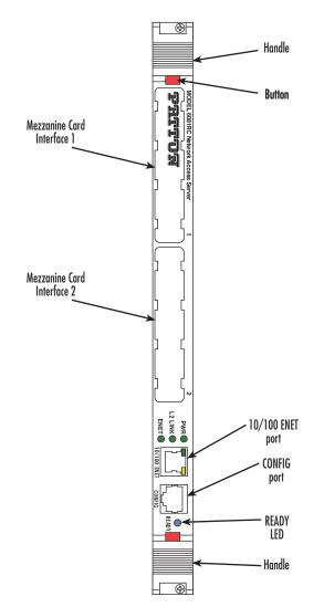
Figure 7. Model 6081RC network and configuration ports
